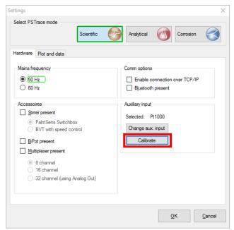
The 'Calibrate' button is enabled if an instrument is connected
