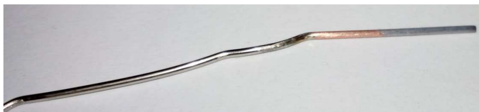
Figure 4.5: steel paper clip covered with zinc for half of the copper part
